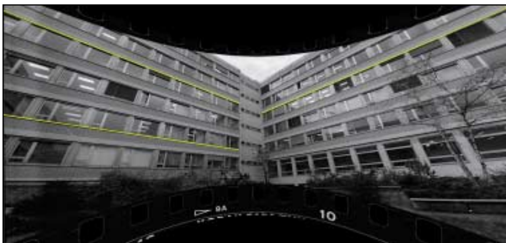
Figure 7: Resampled photograph of a test field. The lines from the test field are depicted as lines in the photograph as well; thus we have a central perspective photo.
