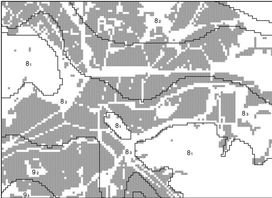
Figure 20: Microseismic earthquake regions and the built-up areas in the central part of Ljubljana. Grid units are 50 m × 50 m. This is a typical example of a map from our Geographical Information System.
