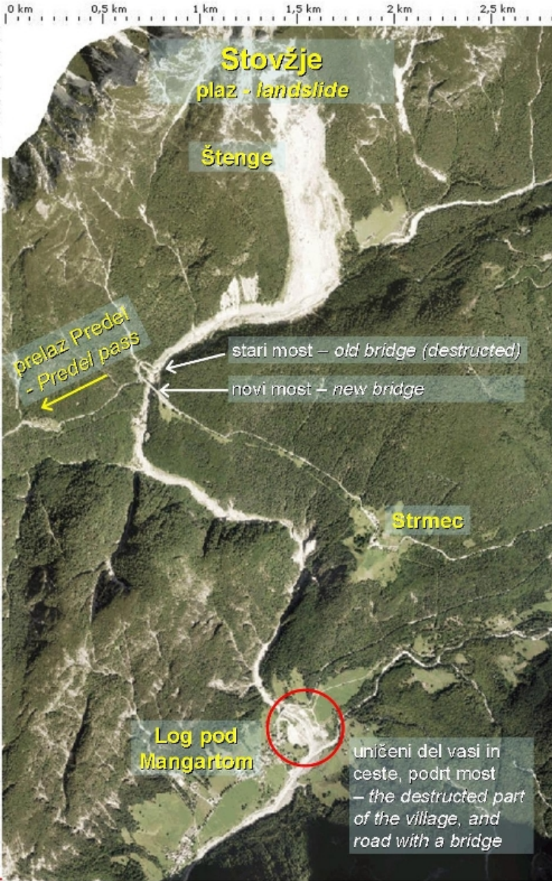
Plaz Stovžje, pot drobirskega toka in del mesta akumulacije; Stovžje landslide, debris flow path and part of the accumulation area;
